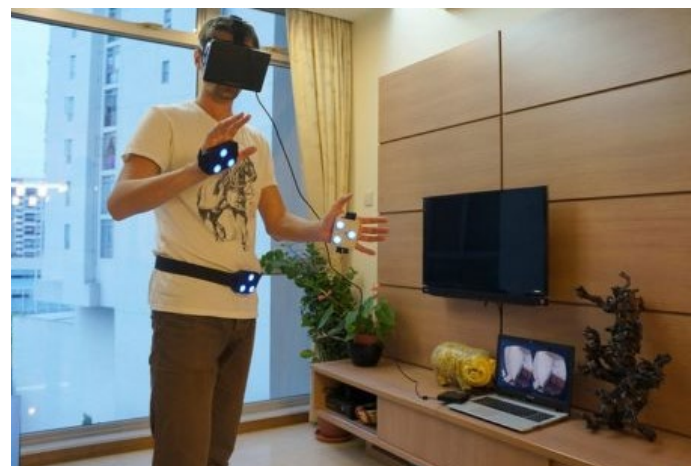
Figure 2-1 iMotion is a motion controller that creates haptic feedback by hand-and-arm interactions through a “virtual touchscreen” [35]
