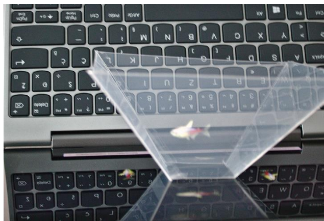
Figure 2-13 Example of pyramidal hologram
