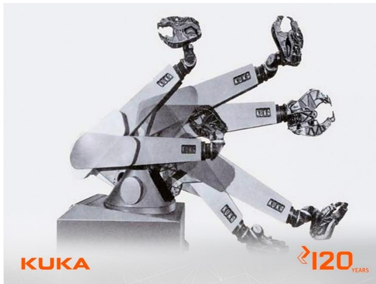
Figure 2-36 FAMULUS industrial robot [123]
