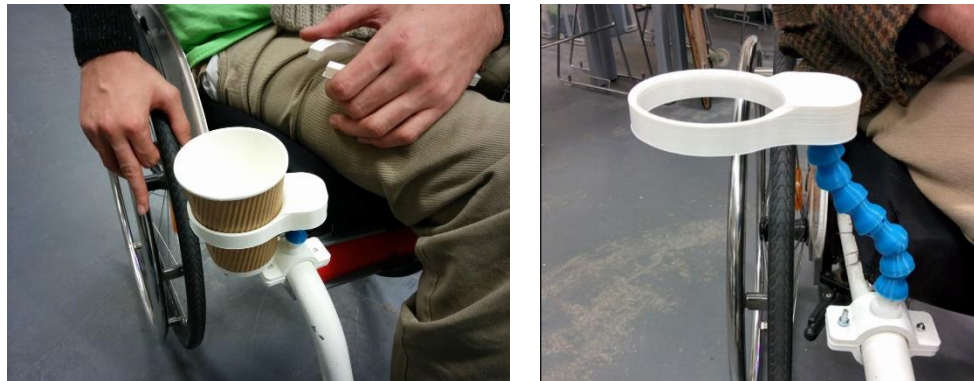
Figure 4-23 Wheelchair cup holder with customizable ball socket joint [306]
