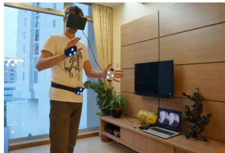
Figure 2-1 iMotion is a motion controller that creates haptic feedback by hand-and-arm interactions through a “virtual touchscreen” [29]
