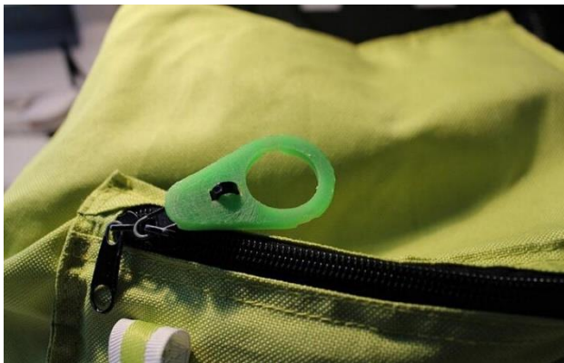
Figure 4-21 3D-printed zippers to be attached to a smaller zipper tab [306]
