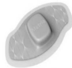
Metria™ Informed Health 3-axis accelerometer, Galvanic Skin Response, 2 temperature sensors (body, skin)
