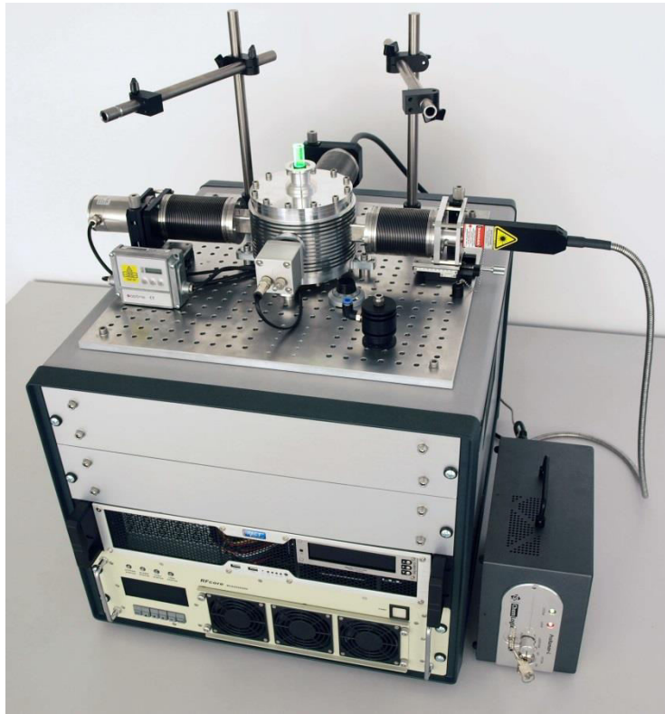
Figure 2. Microwave device for material sintering
